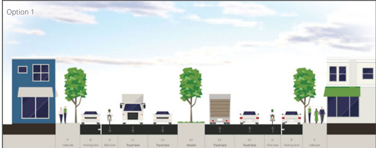
Proposed Typical Cross Section Along E. 14th Street / Mission Boulevard. Option 1 Includes a Class II Bike Lane in Both Directions, Vegetated Median and Sidewalks for Shade, and Preserved On-Street Parking. Source: Fehr & Peers, 2014
