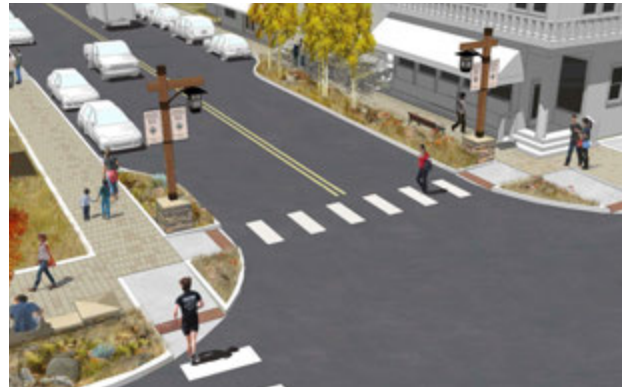
Example of How Curb Extensions (Bulb-Outs) Reduce Crossing Distance, Improve Pedestrian Visibility, and Provide Room for Street Furniture.
