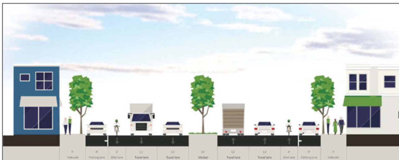
Cross-Section of a Complete Street.
