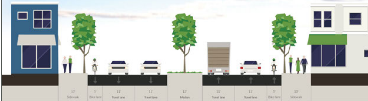
Existing Typical Cross Section Along Lewelling Boulevard Between Hesperian Boulevard and Meekland Avenue Source: Fehr & Peers, 2014
