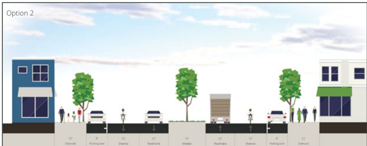
Alternate Proposed Typical Cross Section Along E. 14th Street / Mission Boulevard. Option 2 Includes Two Lane Vehicular Traffic with a Class III (Shared) Bike Lane, Wider Sidewalks to Accommodate Streetscape Improvements such as Shade Trees. Source: Fehr & Peers, 2014
