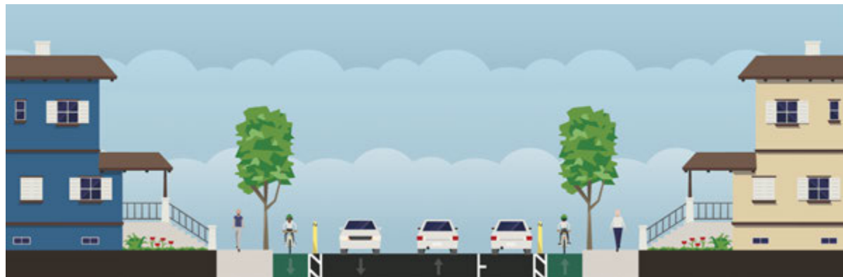
Example of Class IV Bicycle Lane Configuration on a Typical Arterial and Collector Roads. Not representative of actual design or conditions in the ACBD Plan Area.
