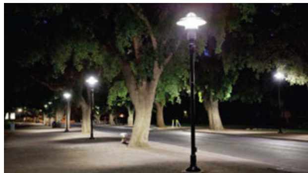
Example of Pedestrian-Scaled Lighting: Shorter Poles Which Serve to Primarily Light the Sidewalk, Improve Visibility, and Sense of Security.
